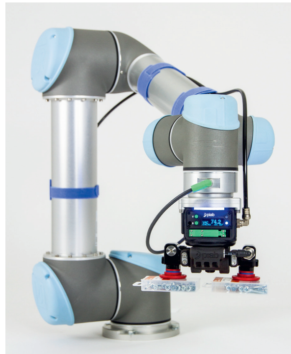
Increased productivity with integrated piSAVE ® Sense valves (object sensing valves), double or single picking of objects.
