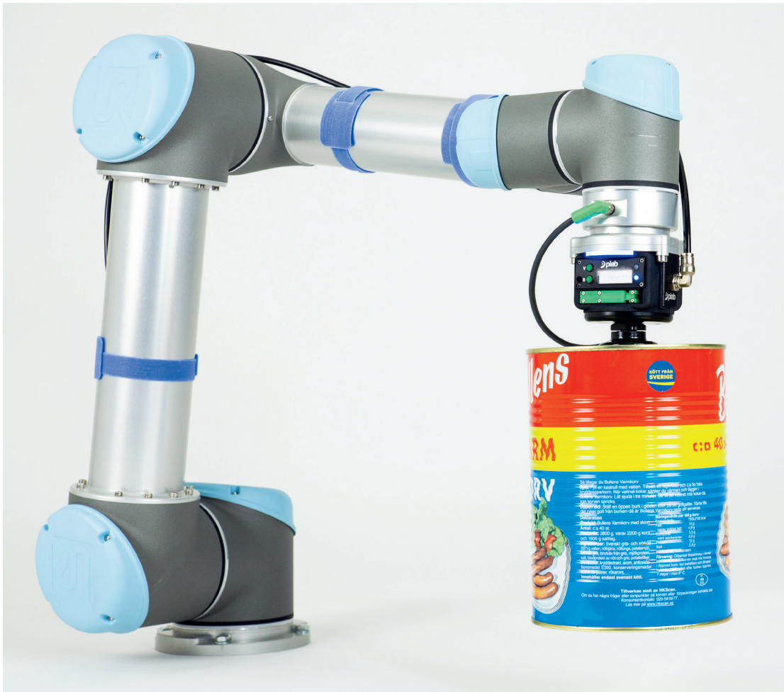
An extended robot arm gripping and moving up to 7 kg [15.5 lbs] object.
